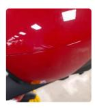
Spoiler Rear Scratched (Painted) Over 25mm Thru Paint Smart Repair
