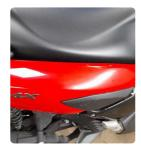
Qtr Panel osr Scratched Over 25mm Not Thru Paint Machine Polish
