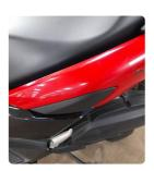
Qtr Panel nsr Scratched Over 25mm Not Thru Paint Machine Polish
